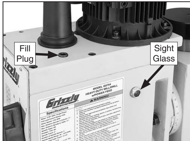
Figure 39. Location of headstock oil sight glass and fill plug.
